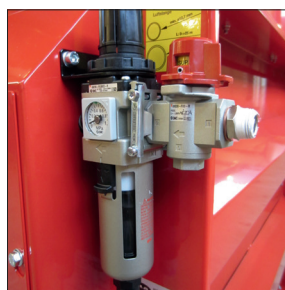
Pneumatic Isolator (Only for Air models)
